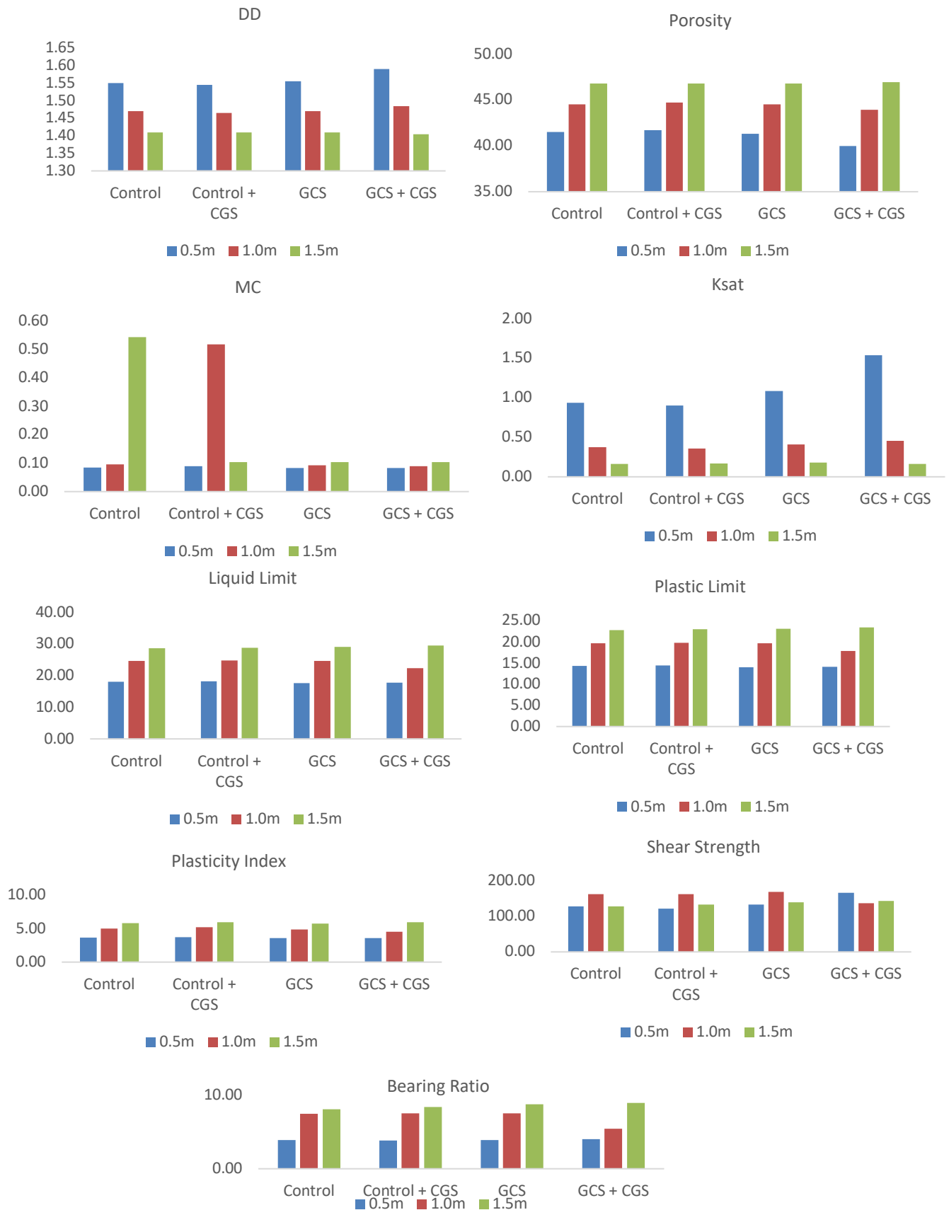
Figure 2.0b: Soil hydro-geotechnical properties as affected by CGS treatment on CS and GCS
